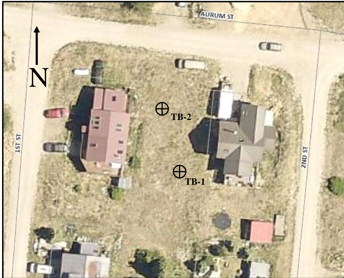
Figure 2.2 Approximate Test Boring Locations
